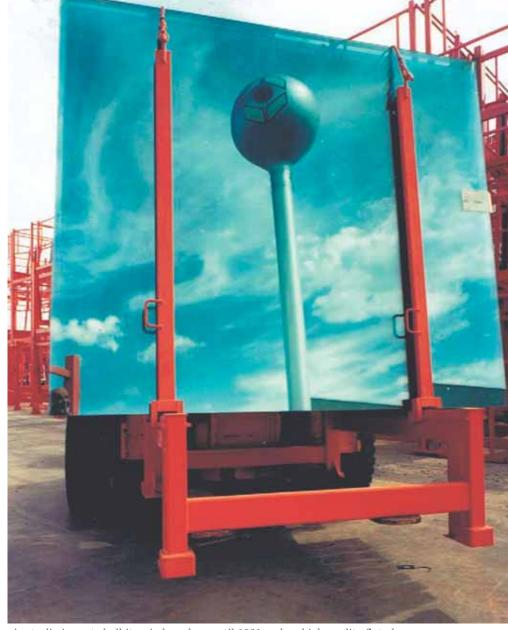
Australia imported all its window glass until 1931 and no high quality flat glass was made locally until 1974. This pallet of Australian-made float glass clearly reflects the water tower at Pilkington ACI's Dandenong plant. Wolfgang Sievers' magnificent photograph was one of a series used to promote the end of 'the wavy window', reflecting on the distortion inherent in the sheet glass which was the only previously made Australian clear window glass
